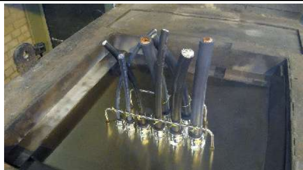
Wölben des Bleches → Rauchaustritt Curving of the sheet → smoke emission Nach ca. 5 Minuten After approx. 5 minutes
