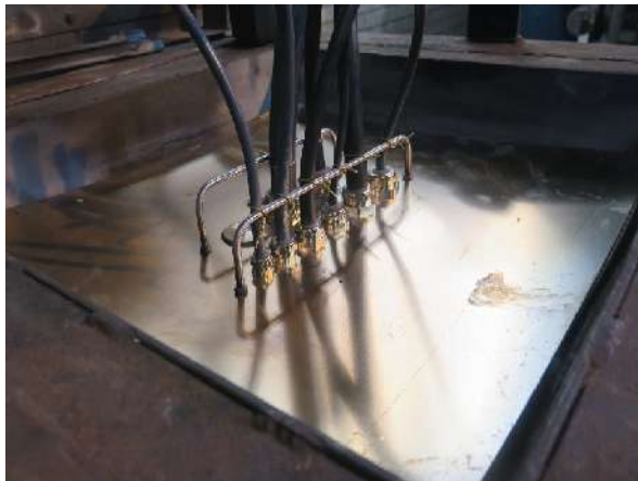
Wölben des Bleches → Rauchaustritt Curving of the sheet → smoke emission
