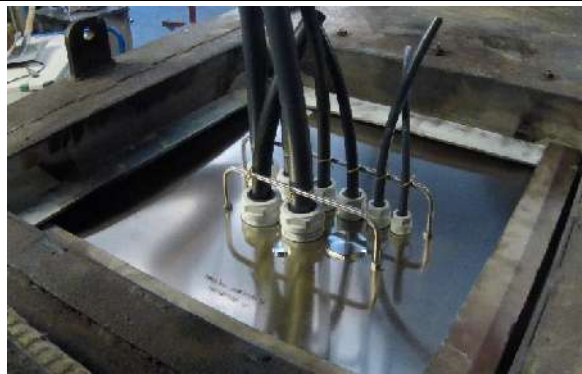
Wölben des Bleches → Rauchaustritt Curving of the sheet → smoke emission
