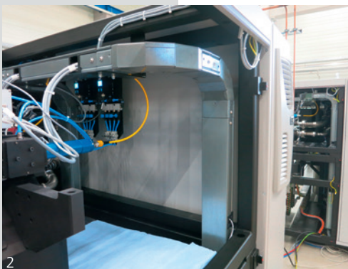
Abb. 2: Der PFLITSCH-Industrie-Kanal in einer Concept Laser M2 cusing Multilaser. (Bild: Concept Laser GmbH) Fig. 2: PFLITSCH Industrial-Trunking in a Concept Laser M2 cusing Multilaser. (Photo: Concept Laser GmbH)
