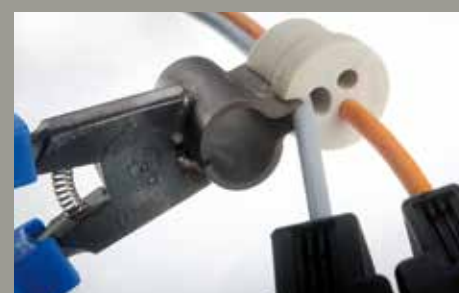
The special pliers allow the cable to be easily fed into the slit sealing inserts.
