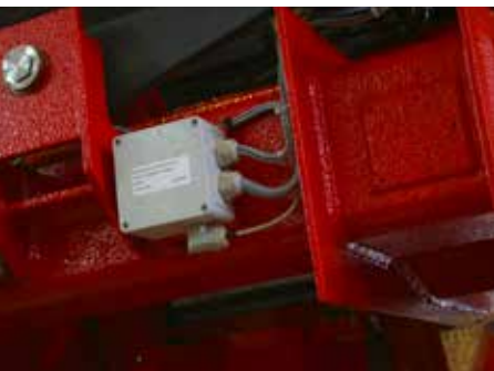
Three variants on a distribution box on the Lafette: Metz installs standard, multiple or elbow cable glands from the UNI Dicht® modular system, depending on the situation. (Photo: PFLITSCH/Lutz)
