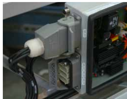
Under harsh conditions of use on the turntable ladder, UNI Dicht® cable glands – seen here in the multiple version with a PVDF cable gland body – provide high ingress protection and operational reliability. (Photo: PFLITSCH/Lutz)
