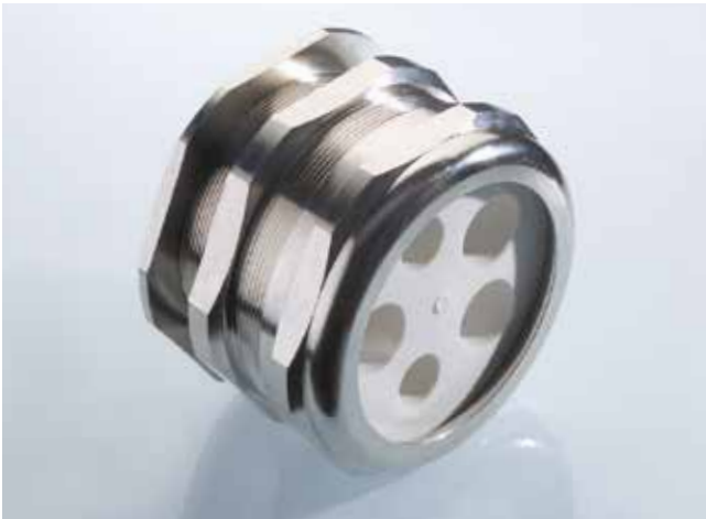
The M120 cable gland from PFLITSCH with its multiple sealing insert allows five power cables to enter the switchgear cabinet in a space-saving and safe manner. (Photo: PFLITSCH)
