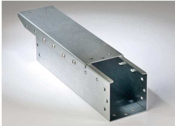
When tested for a customer application in a magnetic-field environment, this combination achieved a screening attenuation of 18 dB compared with an unprotected arrangement of cables. Our standard trunking system, on the other hand, achieved 10 dB attenuation in the same application.
